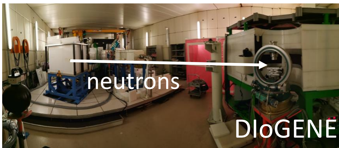
The neutron scattering instrument DIoGENE around the IPHI – Neutrons source.
